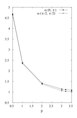
Figure 1. Frequency as a function of temperature for two wave vectors at U = 6 on an  $8 \times 8$  lattice. The continuous line represents the energy at wave-vector  $(0, \pi)$ , and the dash-line the energy at wave-vector  $(\pi/2, \pi/2)$ . We observe that at low temperature (high  $\beta$ ), the dispersion converges. Error bars are smaller than the symbols.
