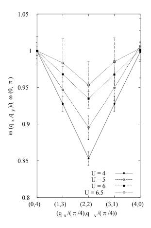
Figure 4. Energy dispersion relation along the  $(0, \pi)$  to  $(\pi/2, \pi/2)$  to  $(\pi, 0)$  line for  $\beta = 3.0$  and t' = -0.35. The coordinates on the horizontal axis must be multiplied by  $\pi/4$ . Each line correspond to a fixed value of U. The dispersion increases with smaller U. Error bars represent the statistical quantum Monte Carlo error.
