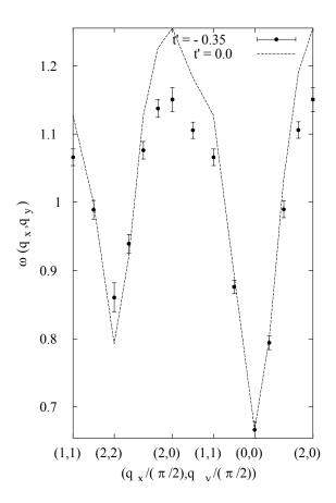
Figure 3. Energy dispersion relation in the SMA as a function of wave vector for  $\beta = 3.0$  and U = 6.0 for an  $8 \times 8$ lattice. The coordinates on the horizontal axis must be multiplied by  $\pi/2$ . The line corresponds to the case t' = 0.0, and the points correspond to the case t' = -0.35. Error bars represent the statistical Quantum Monte Carlo errors.
